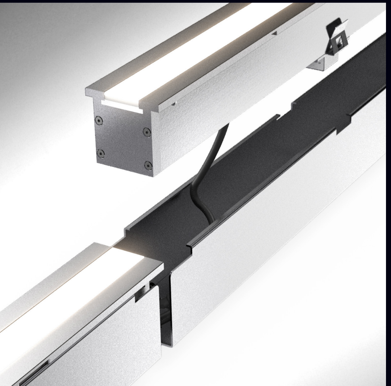
Exploded view - the fixture is installed into the stainless steel housing and held in place with spring clips. The fixture has no visible fixings once installed
