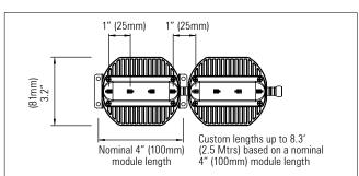
28 x 0.3 Watt medium power LEDs with white reflector per module
